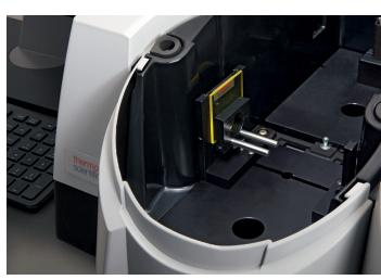
The Solid Sample Slide Holder positions accessories supplied on standard  $2 \times 3$  inch slides. Instrument shown with a Universal Sample Holder and optional second slide holder.
