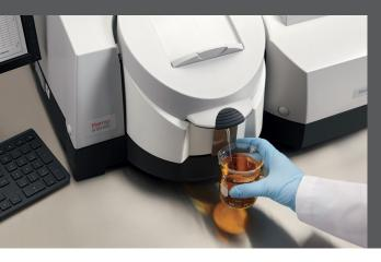
The Evolution 350 UV-Vis spectrophotometer supports Smart Accessories with auto-intelligence. All configurations allow hot-swapping of powered accessories and automatically recognize and initialize each accessory upon installation. Snap the accessory into place and the appropriate software menu for that accessory appears on the screen. Unused accessory software menus are hidden, eliminating possible confusion.
