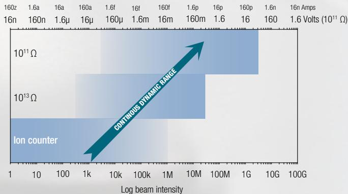
The Triton XT TIMS includes  $10^{11} \Omega$  amplifiers with a 50 V range, as well as  $10^{13} \Omega$  Amplifier Technology and an SEM ion counter, spanning the dynamic range from 1 cps to 30 Gcps.
