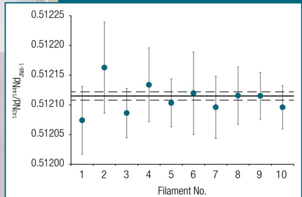
**Results for Nd isotope measurements on 100 pg JNdi-1 aliquots (blue dots with 2 SE error bars).** Solid and dashed black lines refer to the average and 2 SD uncertainty values for published JNdi-1  $^{143}\text{Nd}/^{144}\text{Nd}$  ratios on Nd loadings being 1,000 to 10,000 times higher. Note: the data presented are not warranted because they exceed product specifications.
