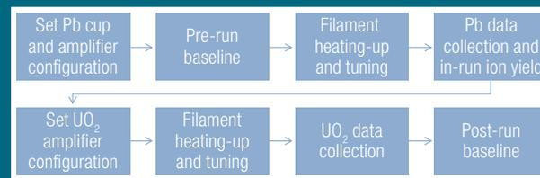
Optimized workflow for the U/Pb measurement, with switchover between the Pb and  $\text{UO}_2$  measurements
