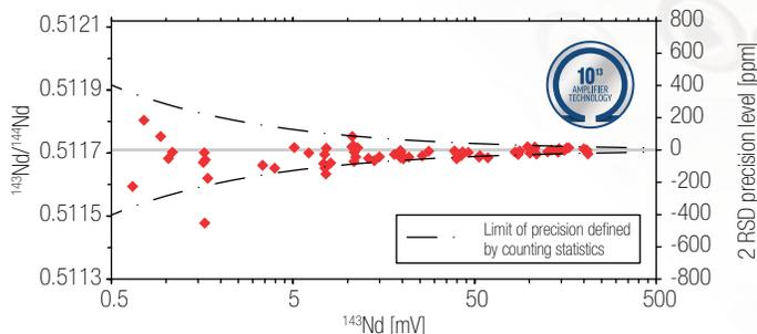
**The isotope system of neodymium (Nd) demonstrates the precision and accuracy of 10<sup>13</sup> Ω Amplifier Technology with gain calibration.**
