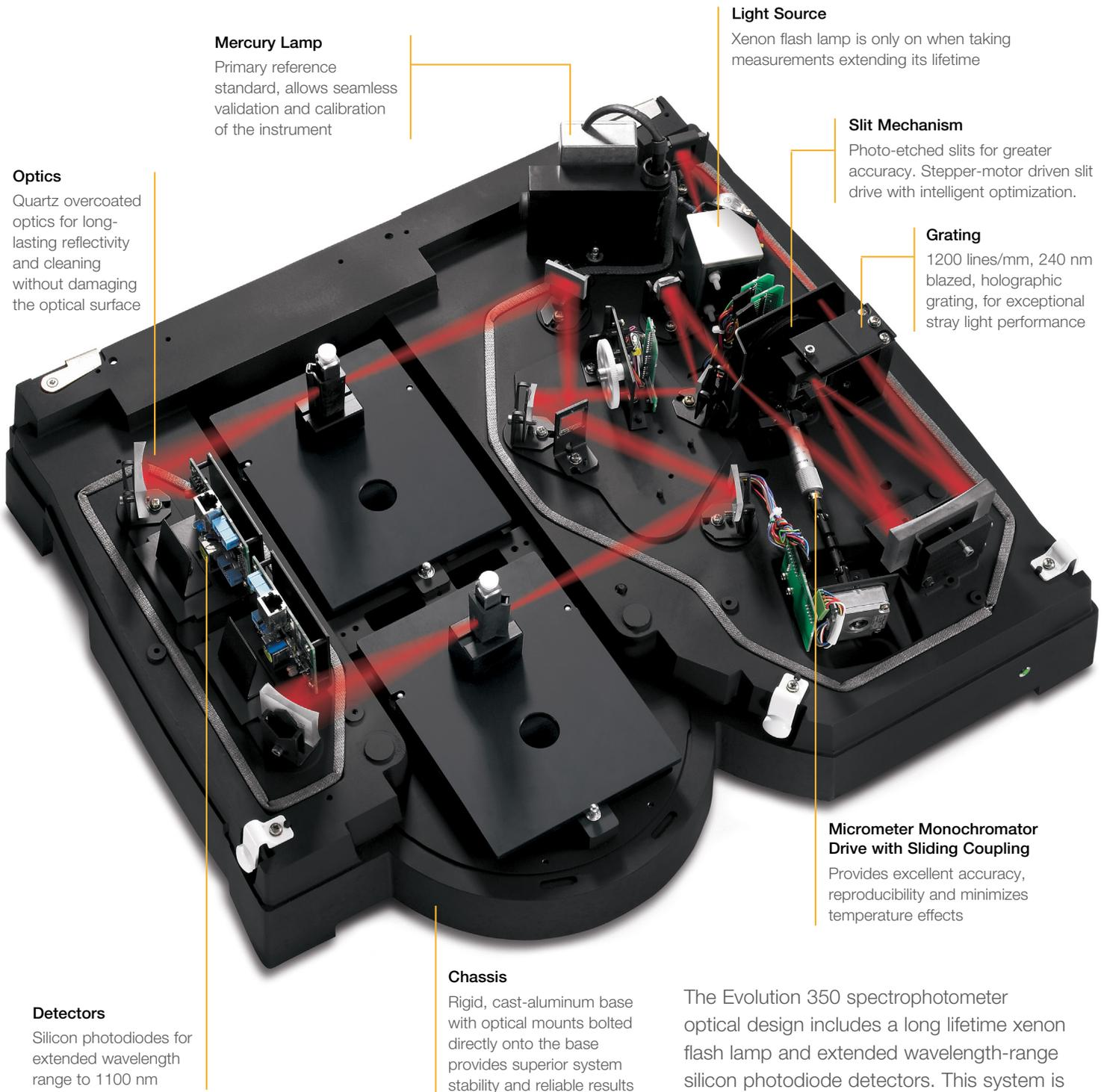
The Evolution 350 spectrophotometer optical design includes a long lifetime xenon flash lamp and extended wavelength-range silicon photodiode detectors. This system is an excellent choice for routine and research laboratories in the Life Science and Pharmaceutical markets.
