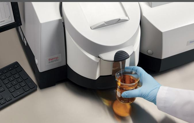
The Evolution 350 UV-Vis spectrophotometer supports Smart Accessories with auto-intelligence. All configurations allow hot-swapping of powered accessories and automatically recognize and initialize each accessory upon installation. Snap the accessory into place and the appropriate software menu for that accessory appears on the screen. Unused accessory software menus are hidden, eliminating possible confusion.
